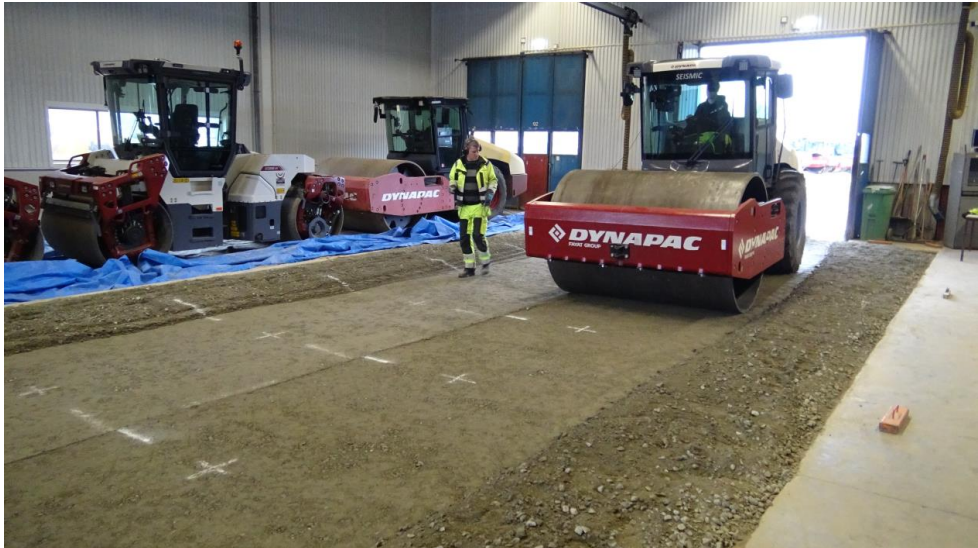
Fig. 1. Test bed and roller in operation.
